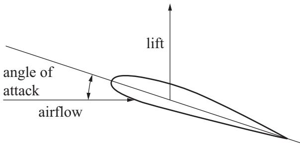
As the speed of the aircraft decreases, the angle of attack,  $\alpha^\circ$ , increases to get more lift. The amount of lift depends on a quantity known as the *lift coefficient*,  $C$ .
